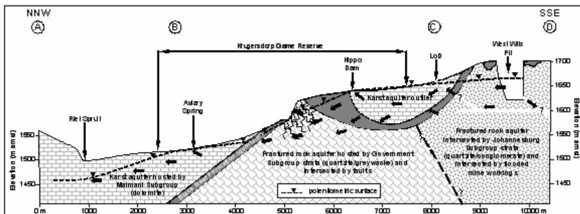
Figure 3: Conceptual hydrogeologic cross-section along the Tweelopie Spruit showing the potentiometric surface from the West Wits Pit in the south to the Riet Spruit in the north.
