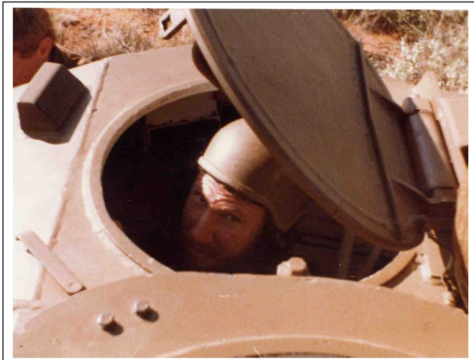
**This image shows the confines of a turret in an Eland 90 where space is at a premium. Note the periscope in front of the gunner's hatch – his entire world is visible through that narrow instrument when hatches are closed.**
